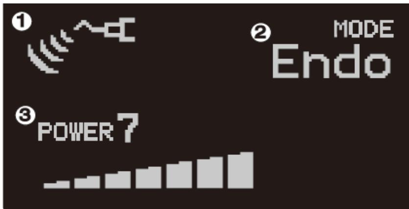
Fig.2 Normal display when using scaler
